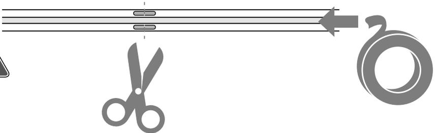
**EN** After cutting the LED strip it is advisable to tape with insulating tape the end of the strip on the cut side, otherwise the resistance to water and moisture will be lost.
